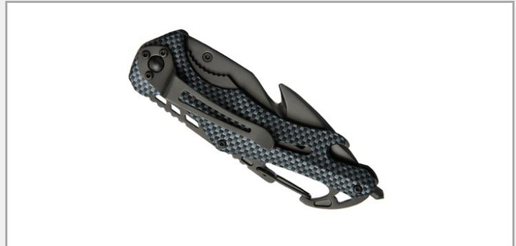
Folding knife with a 420 stainless steel blade with titanium coating. Blade with a fine part (for precision cutting) and a micro-serrated part (for heavy duty task). Anodized aluminium handle in a carbon fiber style. One-handed opening/closing with a Liner lock safety system. Torx screw assembly. Seat belt cutter on the blade and window breaker hammer functions in tungsten carbide at the back of the handle. Bottle opener, carabiner and belt clip. Heather grey RPET pouch included.
